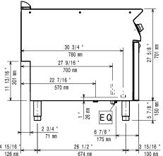
EI = Electrical inlet (power) EQ Equipotential screw Water inlet
